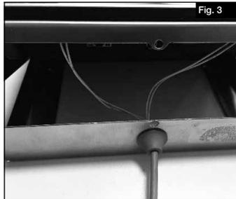
3. Mount the controller in the wall bracket frame and screw the screws (M3) through the following holes, see Fig. 4 (screws M3 included in delivery).
