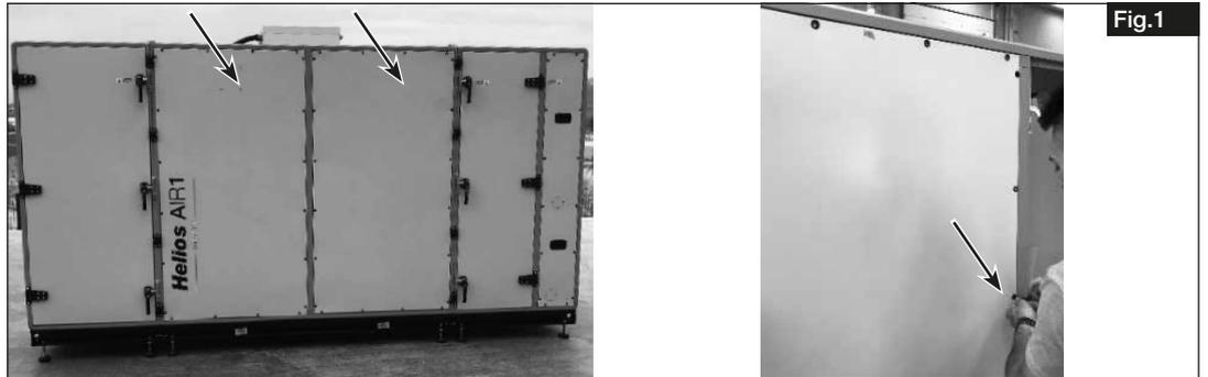
2. Series XHP: Loosen and remove the screws in the service panel and the middle frame, if necessary, see Fig.2.
