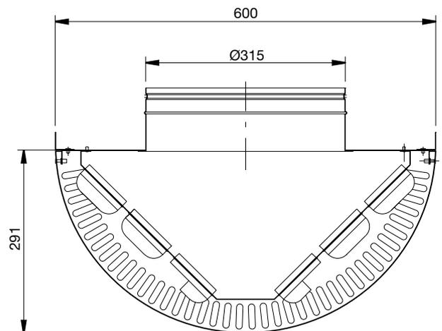
CBAL without plenum box is used, when there is a need for a lower building height. The diffuser is usually mounted directly in an air duct placed above the diffuser. The diffuser is available in a length of 1200, 1800 in addition to 2400 mm with 1 and 2 piece Ø315 connections and 2 x Ø400 connections respectively. The diffuser is also adaptable to most ceiling systems.
